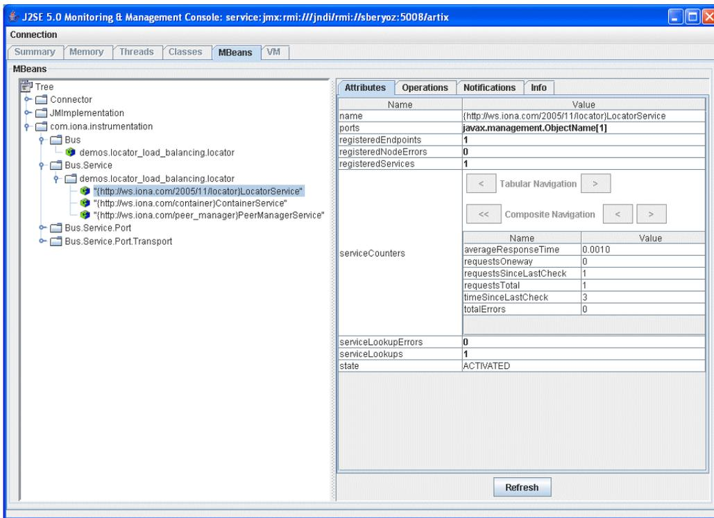
**Note:** When using a JMX console to manage a service running in an Artix container, set the `serviceMonitoring` attribute to `true` to enable service performance monitoring (see “Bus attributes” on page 34).
