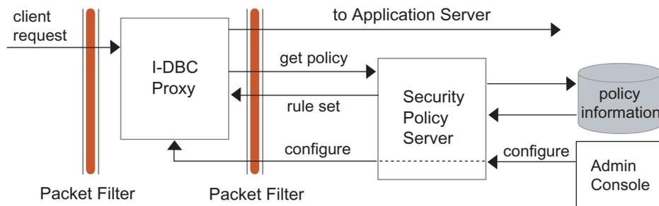
**Figure 1** Separation of I-DBC Components
