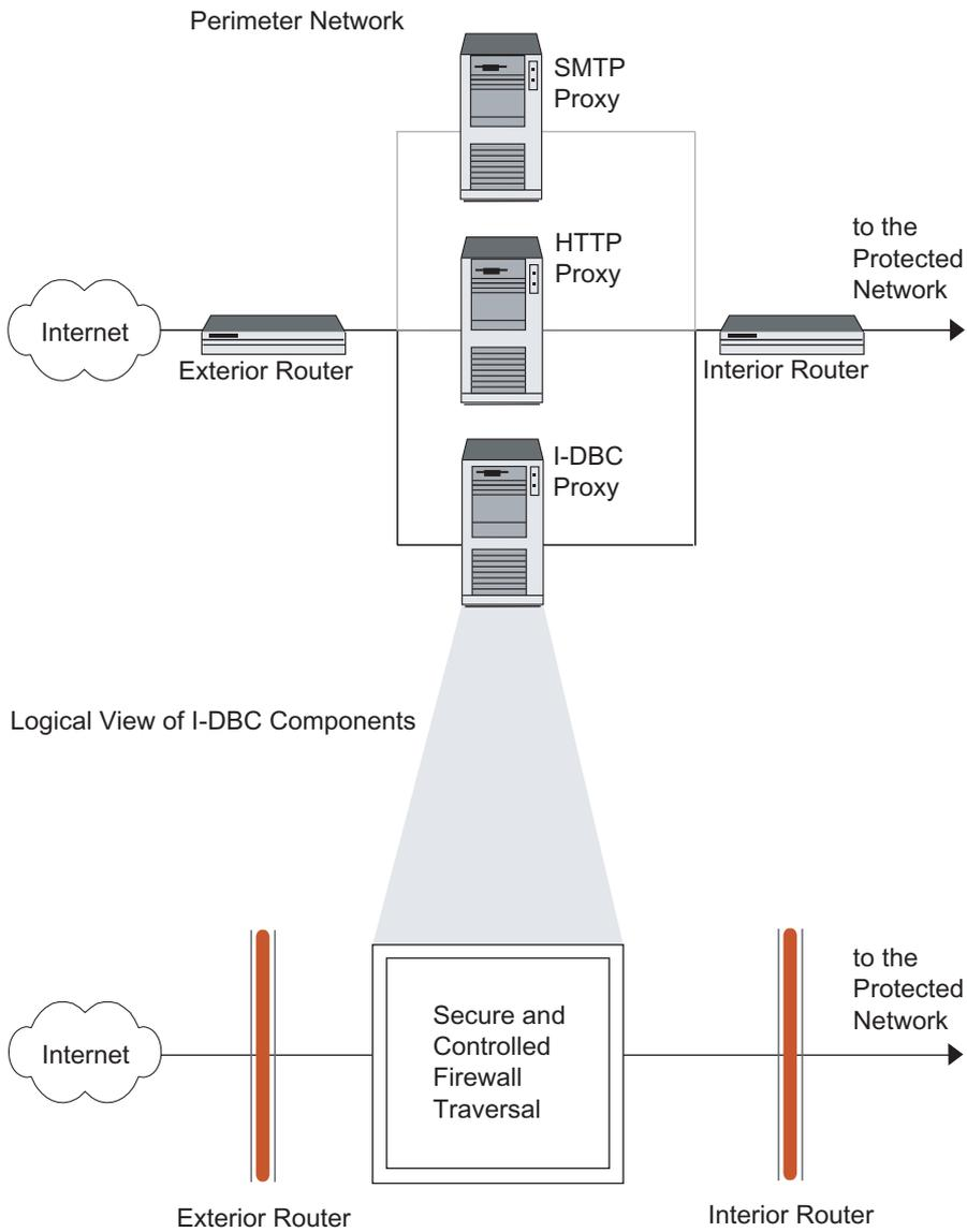
**Figure 2** I-DBC Components in a typical deployment Scenario
