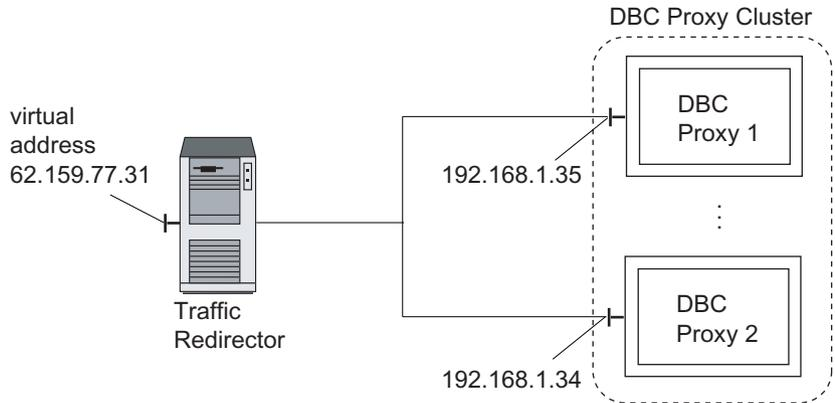
**Figure 30** External Interfaces and Virtual Address of DBC Proxies in a cluster
