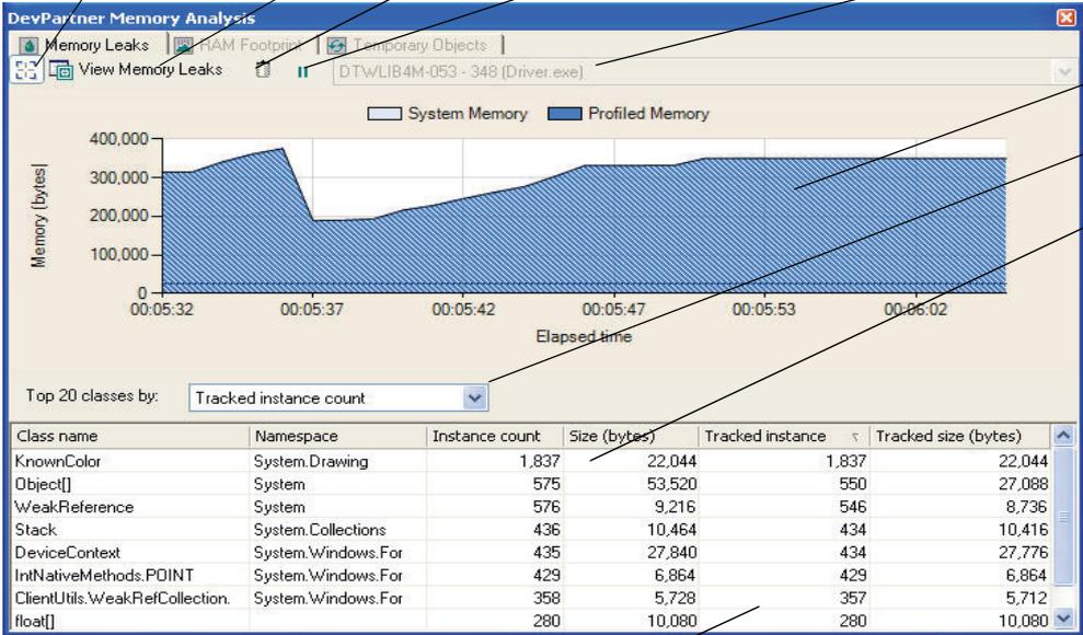
In leak analysis, monitor **Tracked instance count** for objects that were not collected as expected
