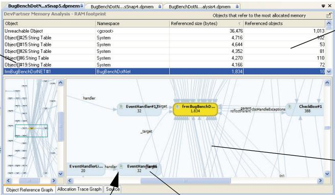
Jump to the allocating source line from any method or object to edit source code
