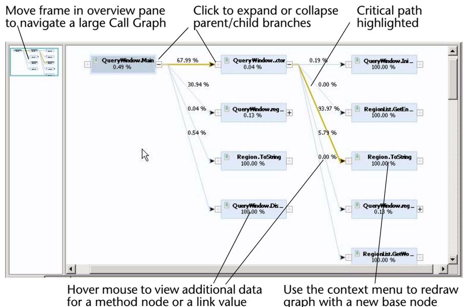
**Figure 5-11.** A Call Graph for an Entry Point Method Shows the Critical Path.
