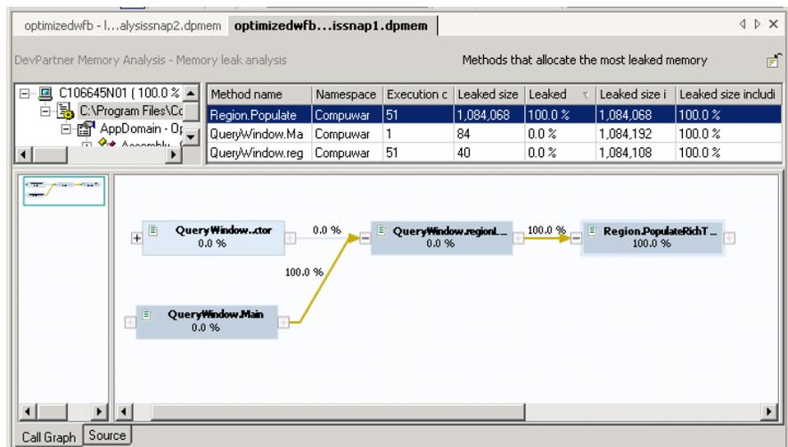
Figure 5-9. Details for Methods That Allocate the Most Leaked Memory.
