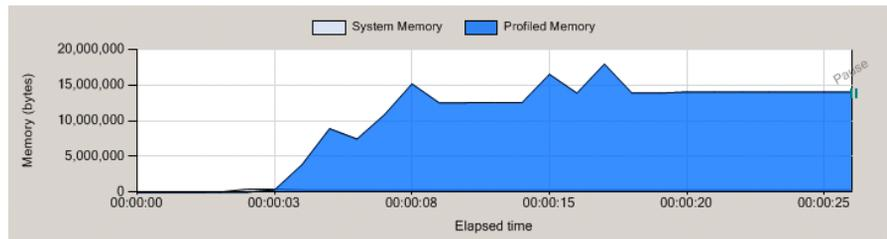
**Figure 5-10.** Real-time Graph Showing a Pattern That Suggests Excessive Temporary Object Creation
