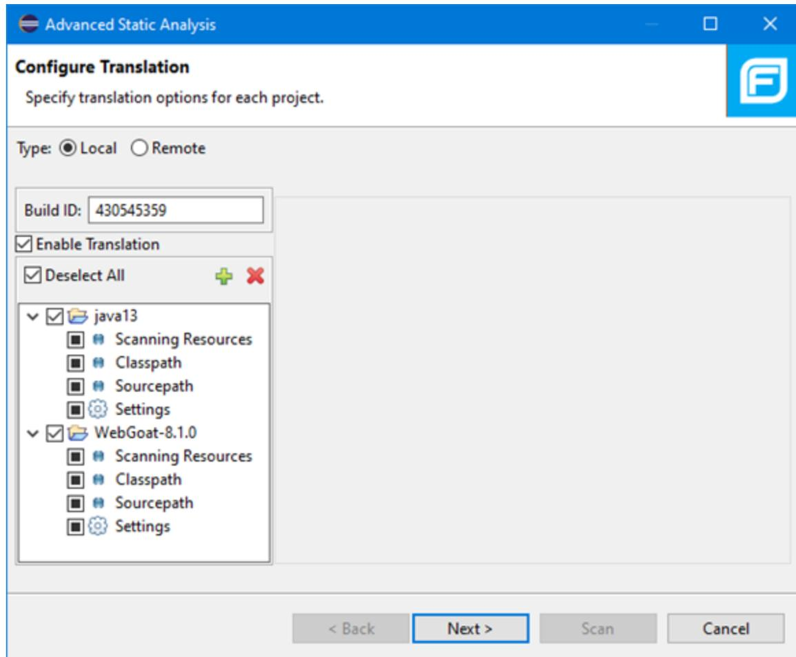
The selected Eclipse projects to be scanned are listed in the left pane. To exclude a project from the advanced analysis, clear the check box for the project.
