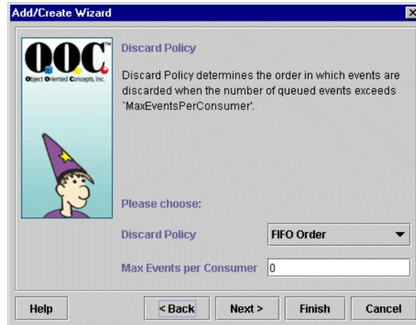
The initial wizard dialog is displayed by invoking the **Create** operation on a selected object. The wizards provide instructions related to the setup of various objects within Orbacus Notify.
