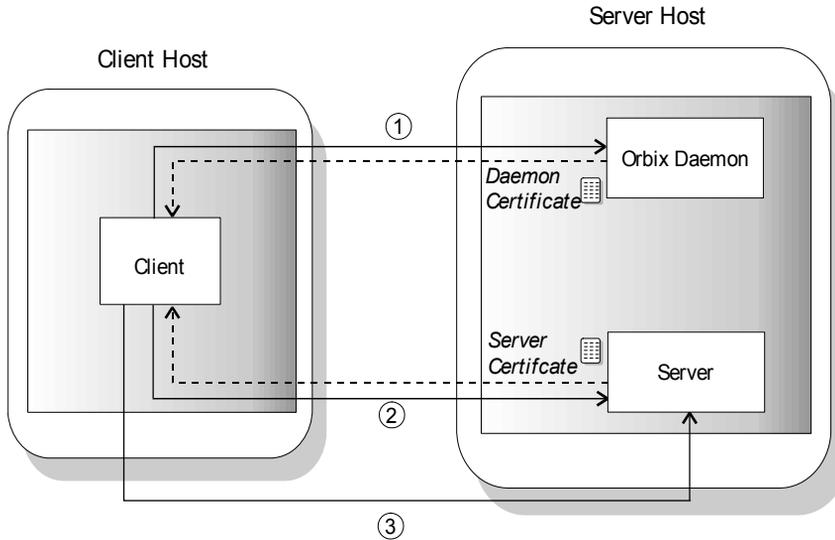
**Figure 2.2:** *Running the Grid Application with SSL Security*
