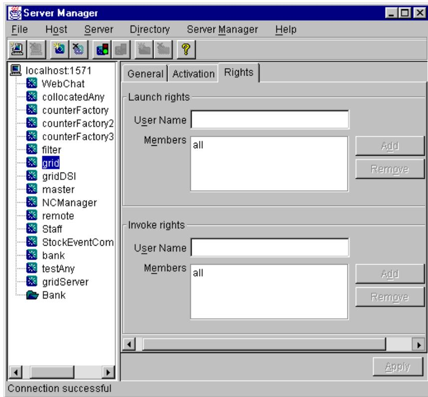
**Figure 14:** *Providing Server Access Rights*
