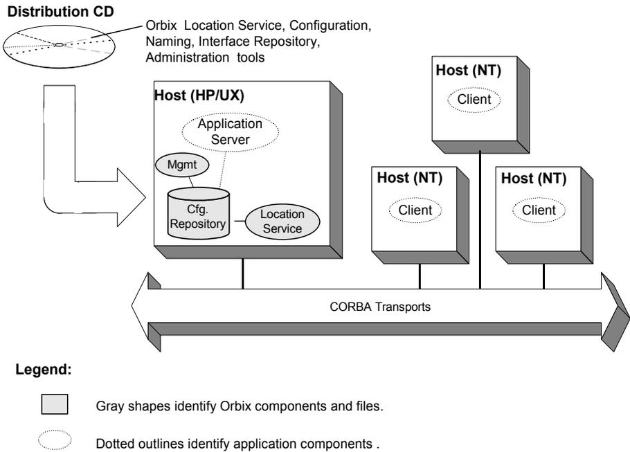
**Figure 10:** *Orbix Environment with Centralized Configuration*
