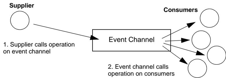
**Figure 2:** *Event Propagation in a CORBA System*
