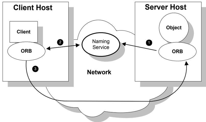
**Figure 4:** Overview of a Simple Orbix Application
