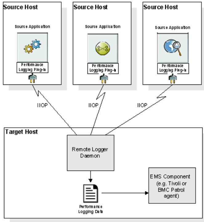
Figure 13: Remote Logging Framework
