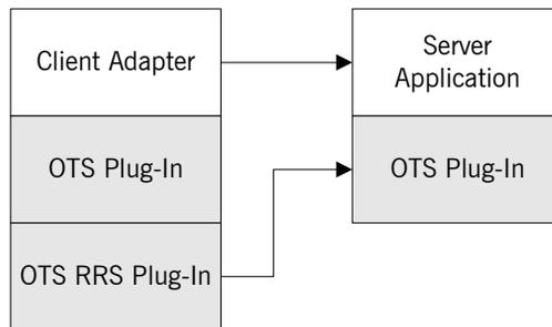
**Figure 20:** Loading the OTS RRS Plug-In into the Client Adapter
