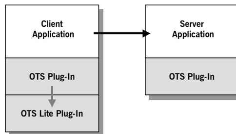
**Figure 18:** *Deployment using the OTS Lite Plug-In*
