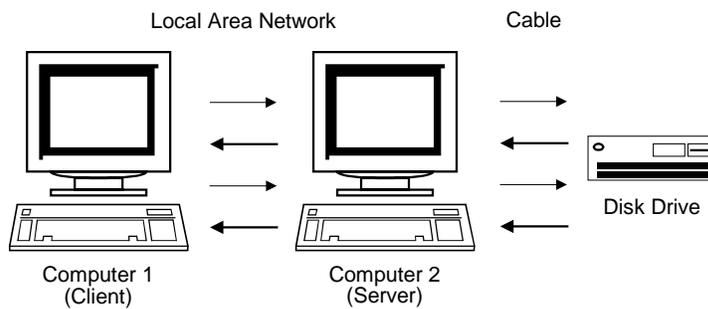
In [Figure 21](#), Computer 2 acts as a conduit, called a server, through which the requests of Computer 1, called a client, are routed. (The server routes requests for more than one client computer, which is an advantage of local area networks.) A more effective way to route requests, however, is shown in [Figure 22](#).
