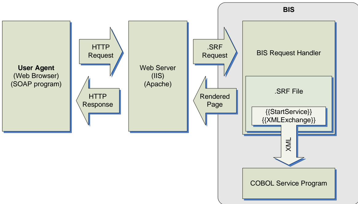
Figure 2-1. BIS Block Diagram.
