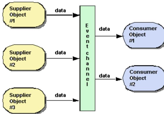
The figure above shows three supplier objects communicating through an event channel with two consumer objects. The flow of data into the event channel is handled by the supplier objects, while the flow of data out of the event channel is handled by the consumer objects. If each of the three suppliers shown in the figure above sends one message every second, then each consumer will receive three messages every second and the event channel will forward a total of six messages per second.
