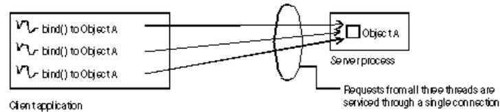
As the above figure shows, all invocations from all threads are serviced by the same connection. For that scenario, the most efficient multi threading model to use is the thread pool model. If the thread-per-session model is used in this scenario, only one thread on the server will be allocated to service all requests from all threads in the client application, which could easily result in poor performance.
