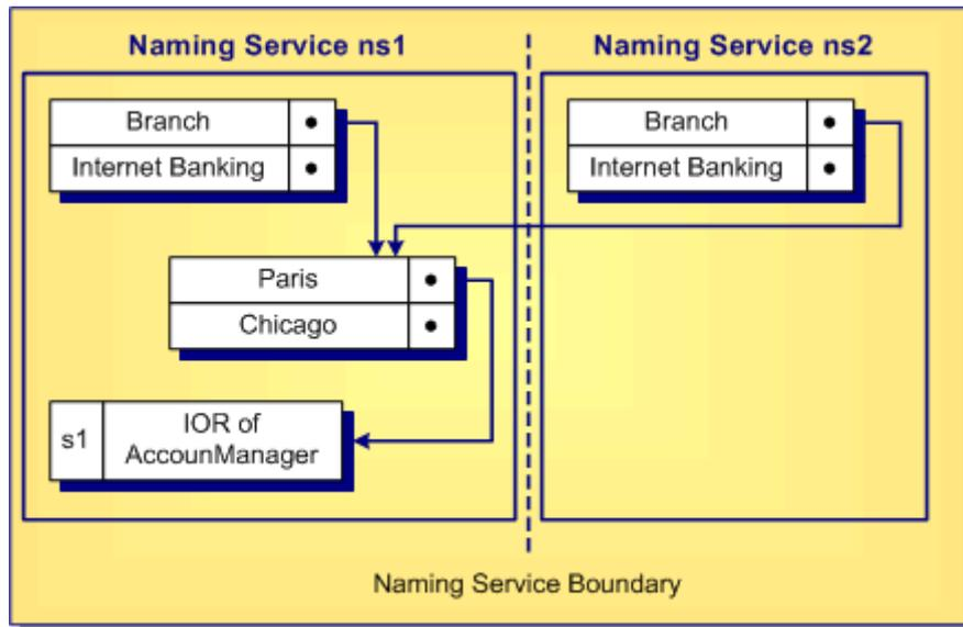
As shown in the figure, the naming context containing `Paris` is bound to `Branch` under naming service `ns1` and also bound to `Branch` under naming service `ns2`. Client can retrieve the IOR of the `AccountManager` object against `s1` either by resolving `ns1: Branch/Paris/s1` or `ns2: Branch/Paris/s1`. In both cases, it gets the same IOR.
