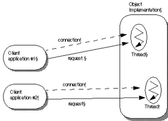
The above figure shows the use of the thread-per-session policy. The Client application #1 establishes a connection with the object implementation. A separate connection exists between Client application #2 and the object implementation. When a request comes in to the object implementation from Client application #1, a worker thread handles the request. When a request from Client application #2 comes in, a different worker thread is assigned to handle this request.
