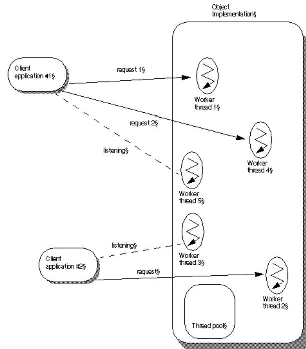
The above figure shows that when a second request comes in from Client application #1, it uses worker thread #4. Worker thread #5 is spawned to listen for new requests. If more requests came in from Client application #1, more threads would be assigned to handle them, each spawned after the listening thread receives a request. As worker threads complete their tasks, they are returned to the pool and become available to handle requests from any client.
