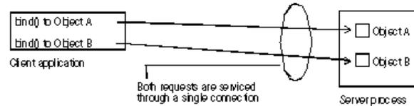
The following figure shows the connections for a client using multiple threads that has several threads bound to an object on the server.
